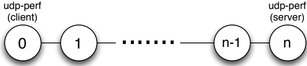
Figure 2: Experimental topology to estimate packet processing rate.
